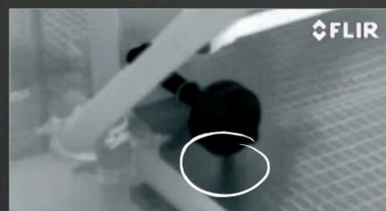
LEAK IS CLEARLY VISIBLE ON THE THERMAL IMAGE
