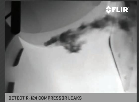
DETECT R-124 COMPRESSOR LEAKS
