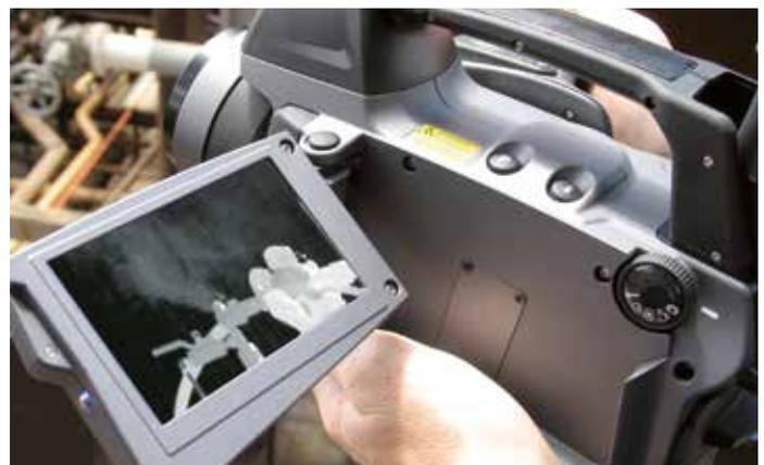
Tiltable, flip-out 4.3" High Contrast Color LCD allows you to view targets more safely from any angle.
